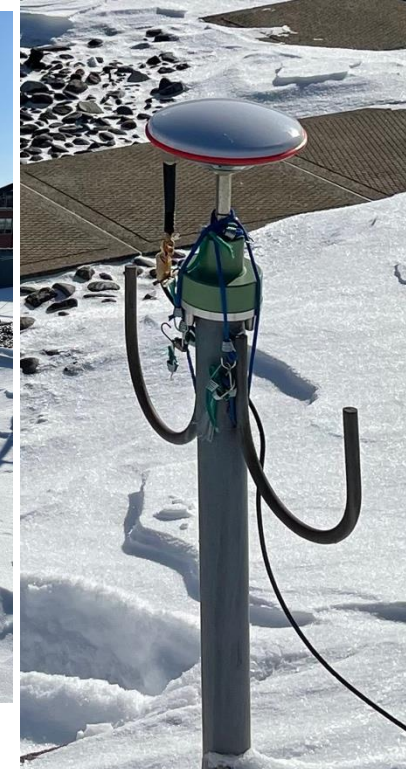
GPS antenna on roof of Gillin Hall
